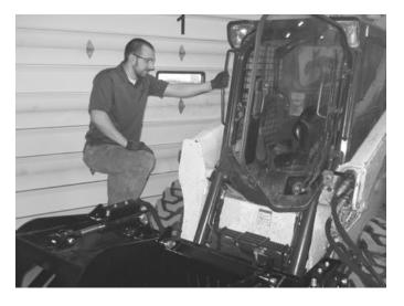
1. Use the step, safety treads, and grab handles to get on and off the loader and attachment.
