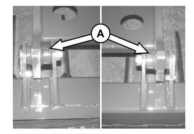
Grease all four cylinder zerks **[B]** every **8 hours** of operation, or more frequently during heavy use.
